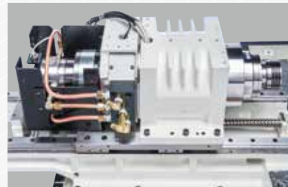
Hydraulic cylinder for main collet chuck (For FS-325/FS-326/FS-327)
