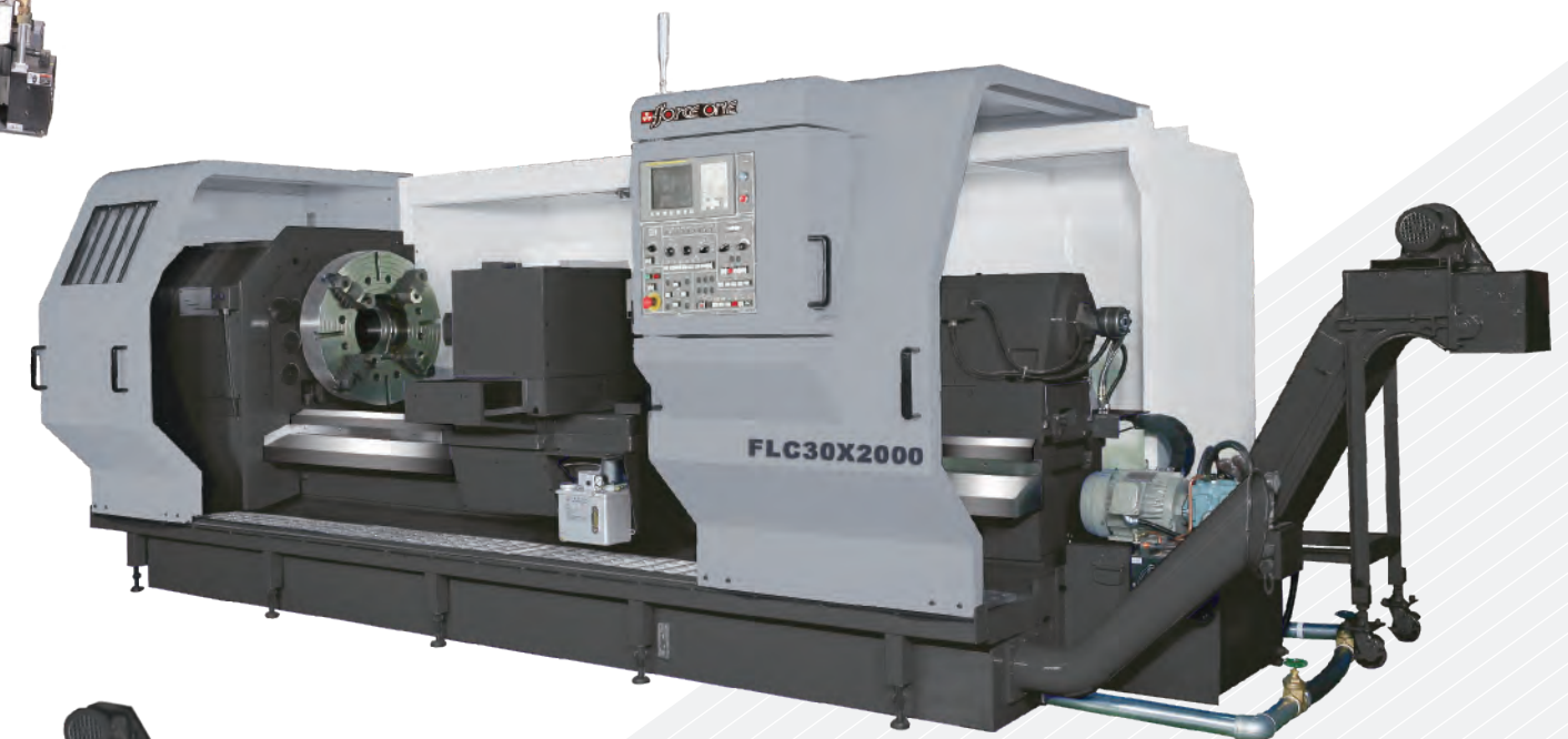
FLC Series: Bed width Auxiliary guide 560 / 710 mm
